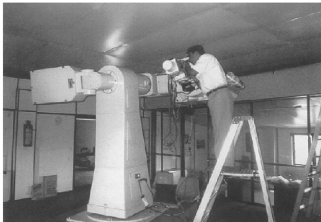
Fig. 2. Sri Lankan astronomer checking and adjusting CCD Camera Spectrograph, plus ST-7 for the reflector, at Arthur C. Clarke Institute [9].
